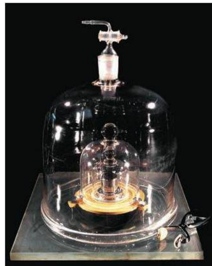
1.4 The international standard kilogram is the metal object carefully enclosed within these nested glass containers.
